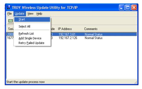
6. When the print server is ready, the firmware upgrade will begin. The IP address of the print server as well as the file you are loading will be displayed.
